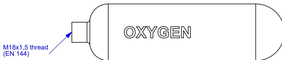
#7183 Tank 2L 300 bar, steel, neck thread M18x1,5, OXYGEN
