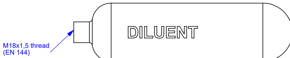
#7182 Tank 2L 300 bar, steel, neck thread M18x1,5, DILUENT
