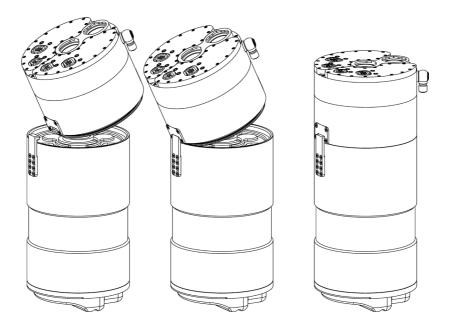
Attach the head to the canister by first inserting the wider opening of the lock on the head of the canister lock lever. Push the head of with your hand so that there is no visible gap between the head and the canister.
