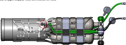
Put the head onto the titanium bracket and screw the medium pressure hose connection to the banjo thread on the head of the unit. Cover the banjo with a plastic cap attached to the hose. Before using for the first time, it is advisable to stretch the cap slightly with your fingers.
