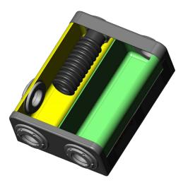
Both counterlungs (inhalation and exhalation) are located in one protective package. The exhalation lung is equipped with a water trap to prevent ingress of water into the head and scrubber. On the side of the exhalation lung is located the overpressure valve (OPV).
