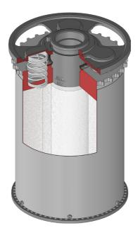
Correct filling of the absorber is described in the CCR Liberty Manual. The procedure does not change. The difference is only for the shortened version of the scrubber, where there is very little difference between the maximum and minimum sorbent levels. Always shake the sorbent properly and always check that the scrubber level has not receded below the minimum mark.
