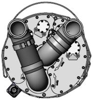
Connect the short connecting hose with the elbows to the head. The elbows are marked by location:
