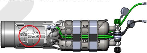
Place the body of the rebreather in the carrier so that both pins on the carrier fit into the openings of the head and the canister. This step is crucial. For safety reasons, It is necessary to carefully check that both pins fit into both holes and the head is secured against disconnection. Disconnecting the head and the canister will cause fatal flooding.
