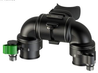
Manual addition valves for oxygen and diluent are placed next to the mouthpiece for better ergonomics and intuitive control. The MAV of oxygen has limited flow to prevent high dose of oxygen at depth.
