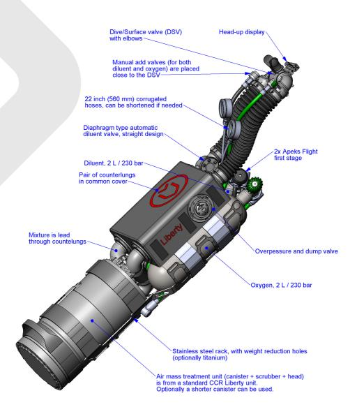
Sidemount CCR is based on CCR Liberty (used air mass treatment unit, electronic systems, DSV, valves, fittings and some others parts).
