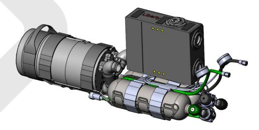
First place the counterlungs on their side so that the OPV is up and towards the front. Connect the left short hose to the bottom port of the counterlung. Tilt the counterlung to the right so that the OPV is on the right and the embroidered logo is at the top. Attach the second hose (it is necessary to turn the port slightly away from you).
