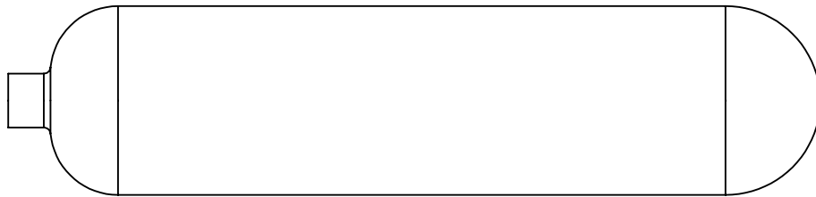
#6111 ECS Steel Cylinder 7 l DIN 144, 230 bar 140 mm diameter, Valve Thread: M25x2
