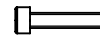
#2208 Screw M4 x 20, socket head, stainless for Handset and HUD (2 pcs used for each)
