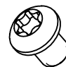
#2248 Button head screw M6 x 8, T30, stainless (for attaching BCD to backplate, 2 pcs used) #2294 Button head screw M6 x 12, T30, stainless (for attaching BCD to backplate, 8 pcs used)
