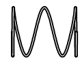
#1526 Additional spring to ADV (increases opening pressure) Not used in CCR Liberty CE
